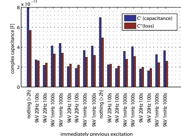
Above: PD measurements (all at 9kV, 10Hz, 200s) on a thermally aged stator coil, with varied frequency of the preceding applied voltage. Measurements and the stated prior excitations were interleaved; the order shown is chronological.
