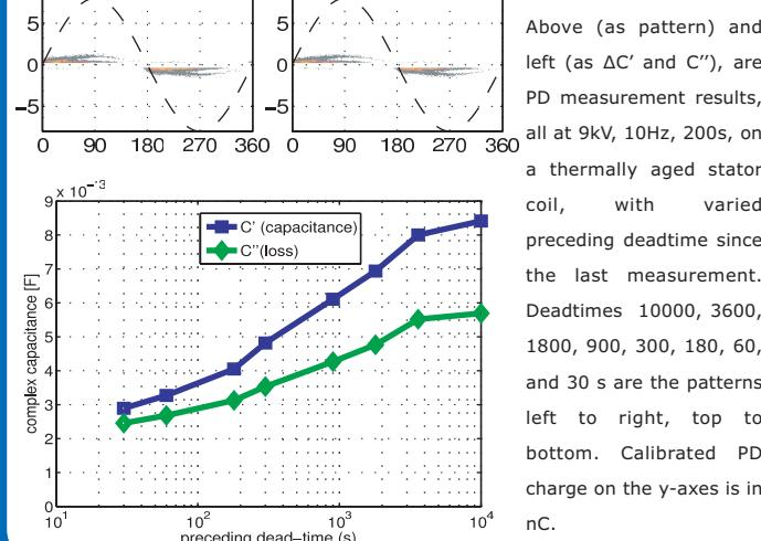
Above (as pattern) and left (as  $\Delta C'$  and  $C''$ ), are PD measurement results, all at 9kV, 10Hz, 200s, on a thermally aged stator coil, with varied preceding deadtime since the last measurement. Deadtimes 10000, 3600, 1800, 900, 300, 180, 60, and 30 s are the patterns left to right, top to bottom. Calibrated PD charge on the y-axes is in nC.
