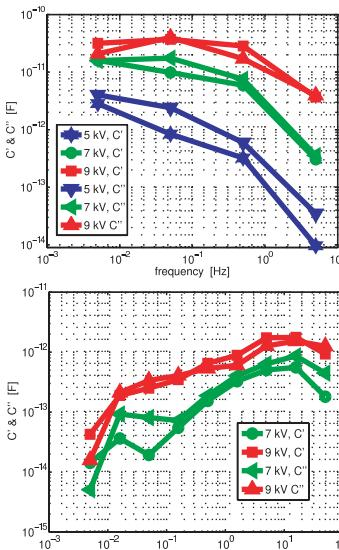
Figures to the left: PD measurements with varied  $V\&f$  on two thermally aged stator coils, as indices  $\Delta C'$  and  $C''$ . Note the different trend in the frequency dependence of these similar objects: different cavities?
