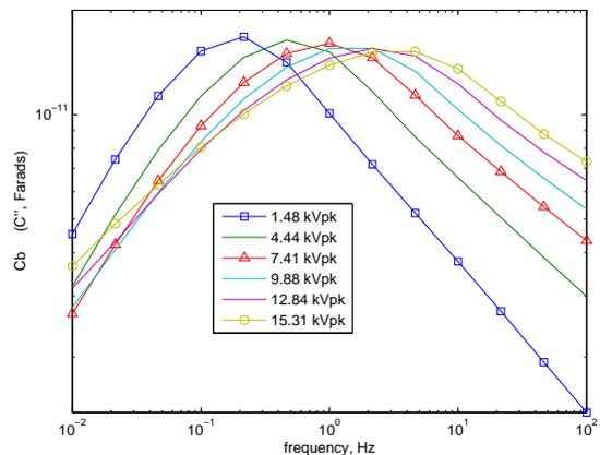
Figure 9:  $C''$  for the taped bar, 1.5 - 15 kV
