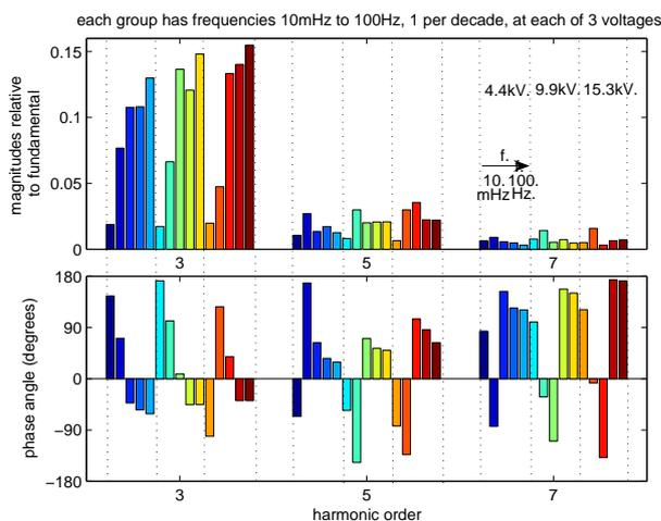
Figure 11: Taped bar, 3rd 5th and 7th harmonics, as proportions of the fundamental component of current. For each harmonic, values are ordered by ascending voltage magnitude then within this by ascending frequency.
