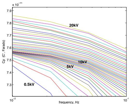
Figure 8:  $C'$  for the taped bar, showing the clustering of low-frequency capacitance at intermediate (5-10kV) voltage levels
