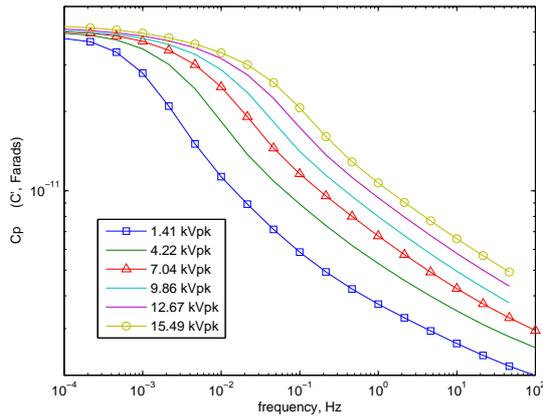
Figure 7:  $C'$  for the painted bar, 1.5 - 15 kV
