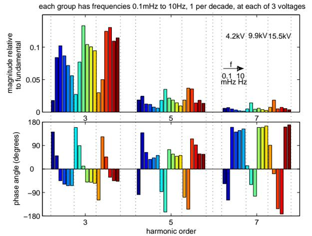
Figure 12: Painted bar, 3rd 5th and 7th harmonics, as proportions of the fundamental component of current. For each harmonic, values are ordered by ascending voltage magnitude then within this by ascending frequency.
