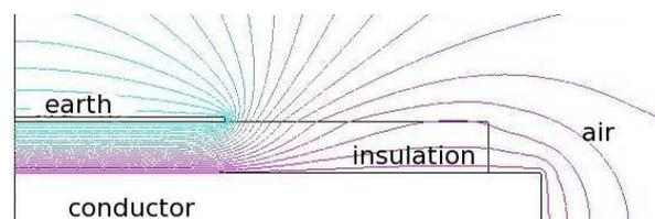
Figure 4: Equipotential lines for the electrostatic case of a high-voltage central conductor, solid insulation, and earthed outer electrode that stops part way along the insulation surface
