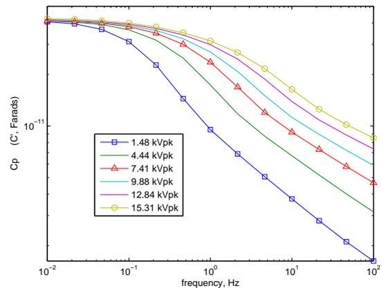
Figure 6:  $C'$  for the taped bar, 1.5 - 15 kV
