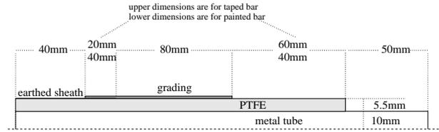
Figure 5: Geometry details of the bars: a symmetric quarter geometry.
