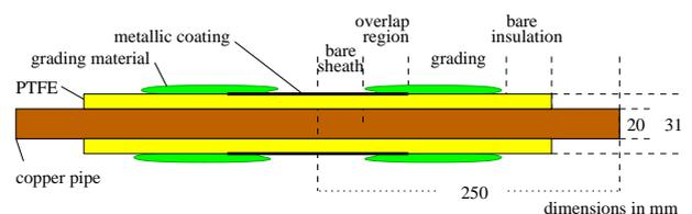
Figure 1: Diagram of the laboratory test-bars used for measuring DR of stress-grading systems
