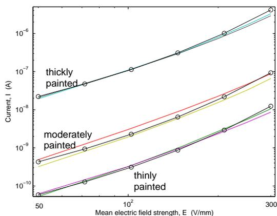
Figure 3: Fitting (marked with circles) of eq. (1) to data from two measurement sequences on each of three sections of paint of different thickness along a 30mm diameter tube.
