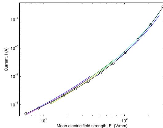
Figure 2: Fitting (marked with circles) of eq. (1) to data from two measurements on each of four lengths (10,20,40,80mm) of half-lapped tape along a 30mm diameter tube.
