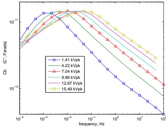
Figure 10:  $C''$  for the painted bar, 1.5 - 15 kV
