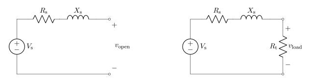
The impedance is estimated by comparing two situations: the open-circuit voltage  $v_{\text{open}}$  (left), and the voltage  $v_{\text{load}}$  with a test-load  $R_{\text{t}}$  connected (right).
